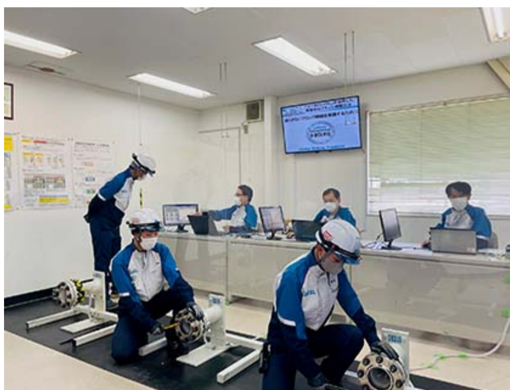
(Photo 2) Simulator-based scientific training for flange tightening
